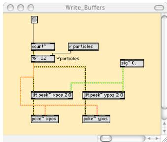
**Figure 2.** Storing matrix values in signal buffers.
